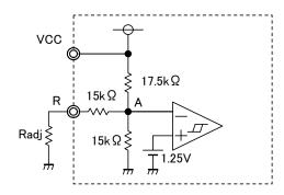
If change Radj, VCC detective voltage is variable.
